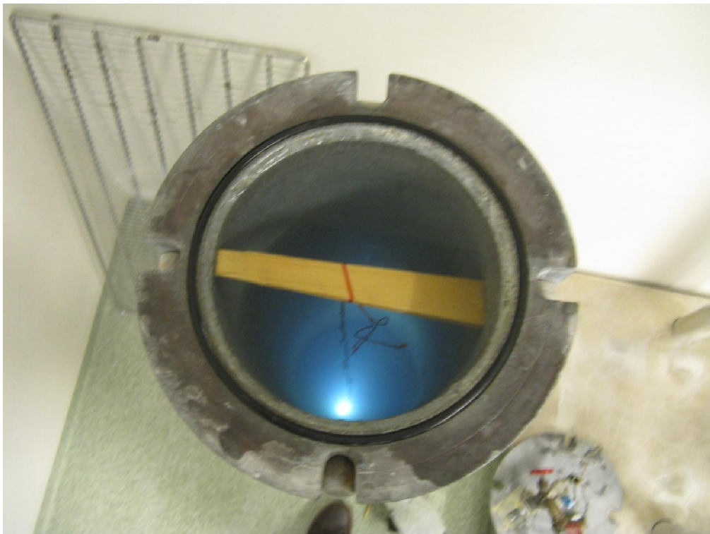
Picture 5: EUT inside the pressure vessel after the IPX8-test.
