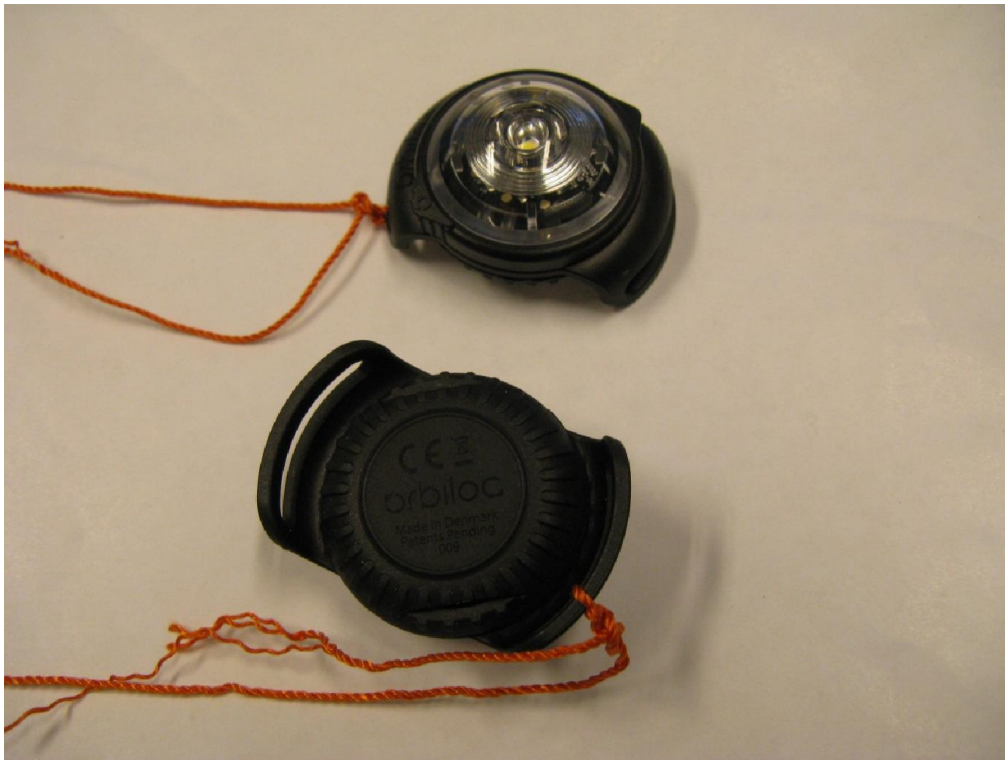
Picture 1: EUT before the IPX8-test.
