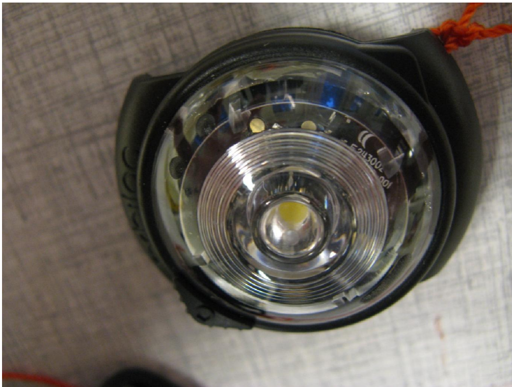
Picture 7: EUT after the IPX8-test; no ingress of water.
