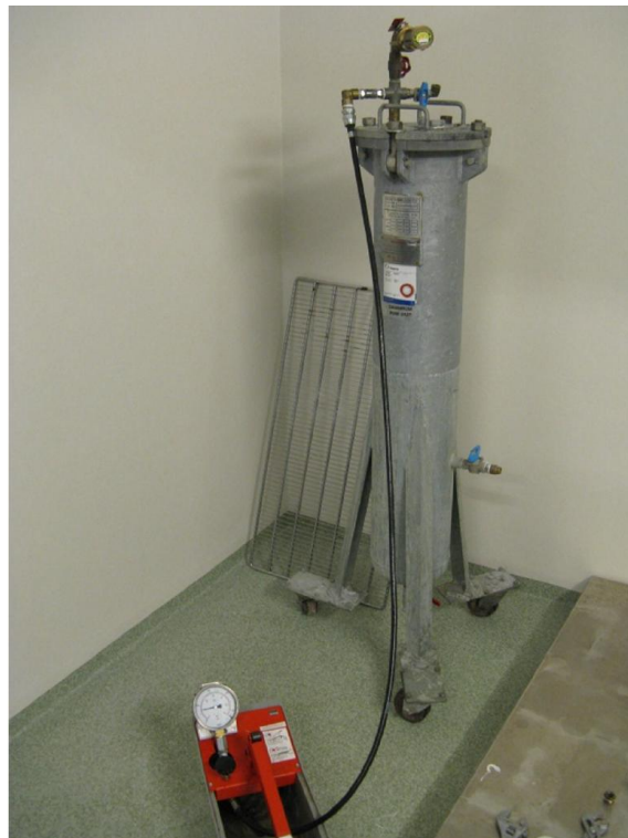
Picture 3: EUT during the IPX8-test.
