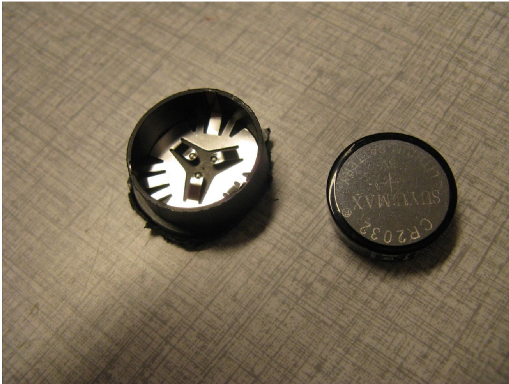
Picture 10: EUT after the IPX8-test; no ingress of water.
